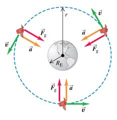
The satellite is in a circular orbit: Its acceleration  $\vec{a}$  is always perpendicular to its velocity  $\vec{v}$ , so its speed v is constant.
