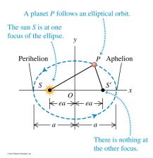
**Figure 5** – The geometry of an elliptical planetary orbit about the sun. The sun is located at one of the foci of the ellipse.
